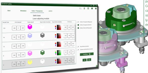
Colours and transparencies from the CAD system ,which cannot be extinguished, are assembly properties. With the toolbox these can be quite simply removed.
